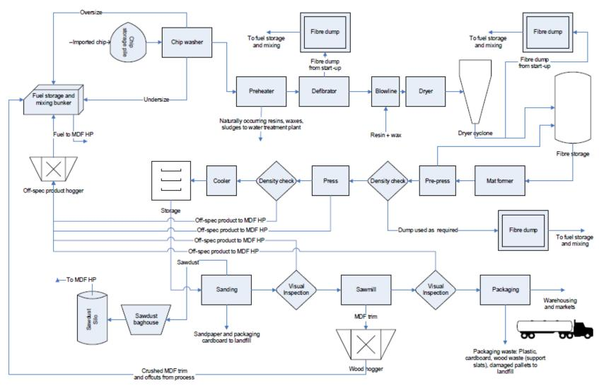
Figure 1 - Schematic Overview of the MDF Production Process
